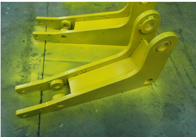
Fig. 11 Image of magnetic arm unit composed of 2 side plates and 1 rib plate used to connect the hydraulic cylinders
