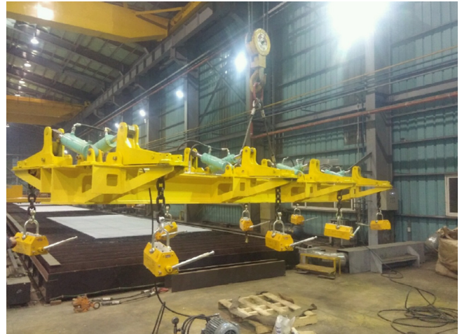
Fig. 12 Image of a assembled hydraulic -magnetic clamp
