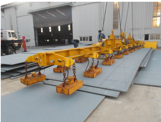
Fig. 2 Actual view of current magnetic crane device
