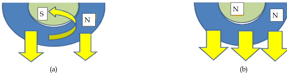
Fig. 16 Schematic image of arrangement in permanent magnet; (a) reverse polarity, (b) same polarity
