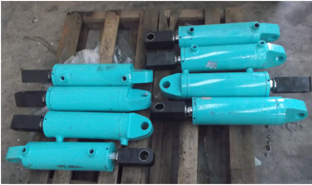
Fig. 10 Image to show the hydraulic cylinder used for the hydraulic, magnetic clamp device
