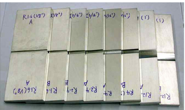
(b) Grooved specimens (Bai and Wierzbicki, 2008)
