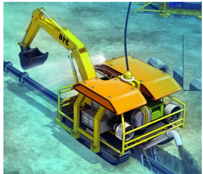
Fig. 1 Underwater Construction Robot
