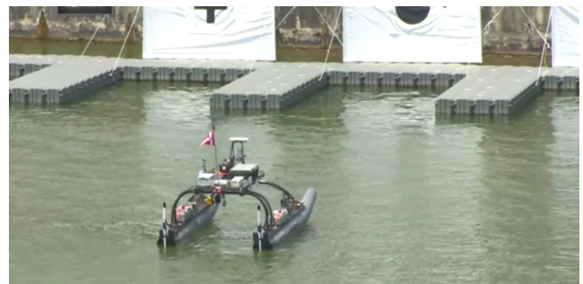
Fig. 1 Example of forward-direction docking of USV (Image Source : Maritime Robotx 2014 USV Competition)
