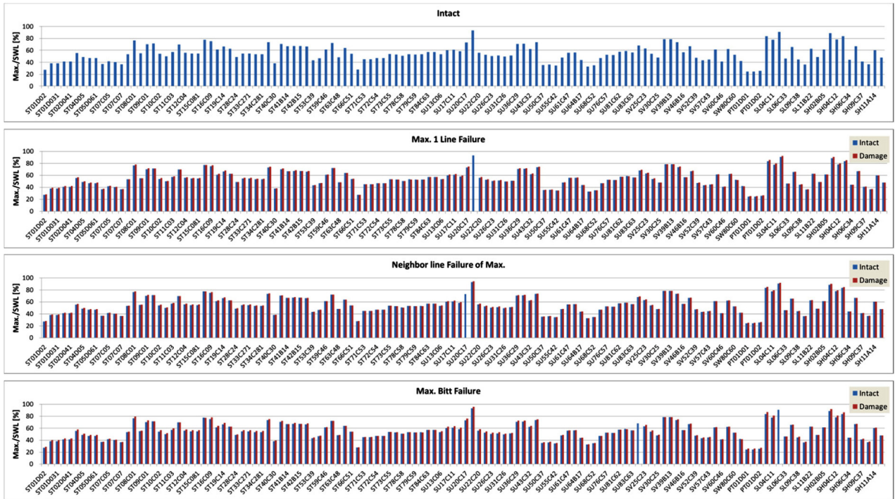
Fig. 10 Mooring analysis results for mooring lines(Intact, Max. 1 line failure, Neighbor line failure of Max. line, Max. loaded bitt failure)
