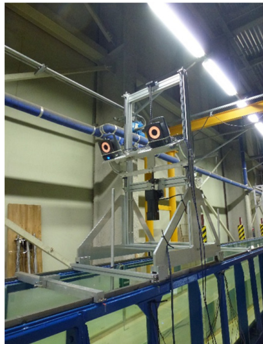
(d) Installed motion capture system with two T40-Cameras
