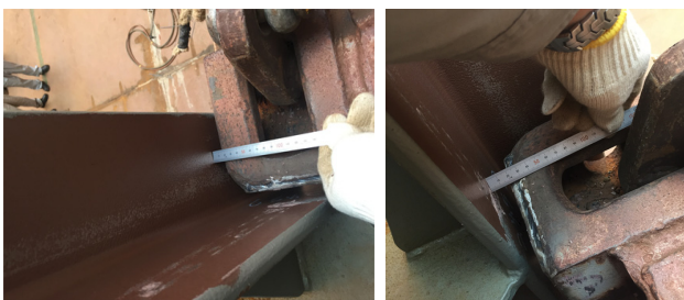
Fig. 13 Interval measurement between cell guide and container box
