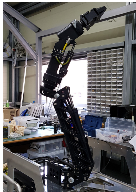
Fig. 2 7E-MINI Manipulator of ECA Group
