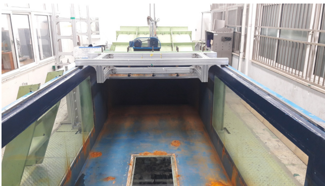
Fig. 1 Circulating water channel (left) & 3-D motion measuring instrument (right)
