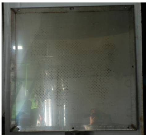
(a) A flat plate-type radiant heat shield
