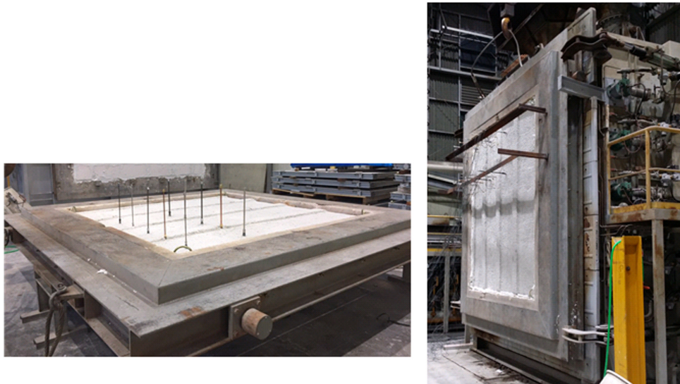
Fig. 6 Actual fire test specimen with spray type insulation(left) and installation on vertical furnace(right)
