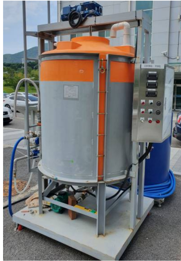
(b) Agitator system (One ton capacity)
