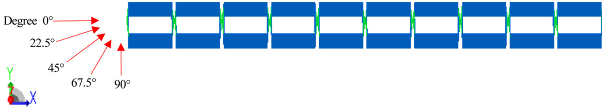
Fig. 3 Floating breakwater and wave direction
