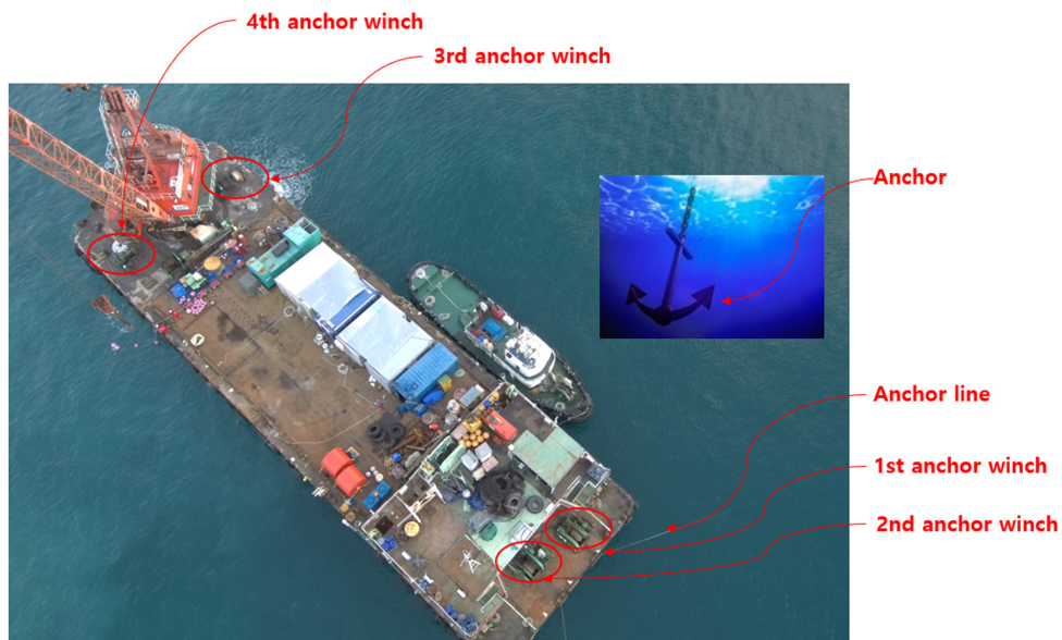
Fig. 4 Barge anchor system
