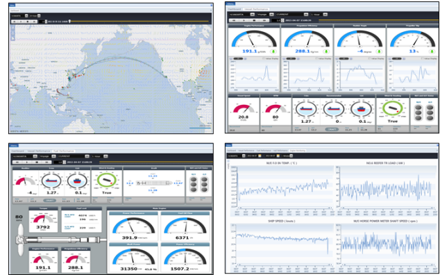
Fig. 7 Photographs of energy efficiency monitoring system (EEMS)
