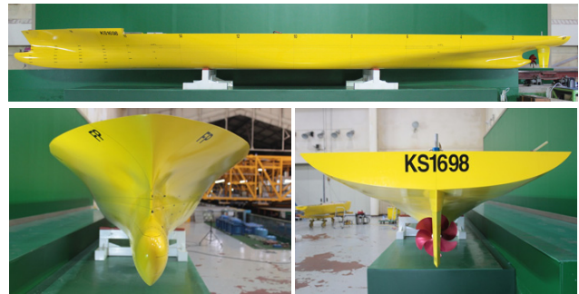
(a) Photographs of model the ship and propeller
