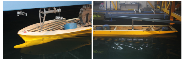
(b) Photographs of the self-propulsion test
